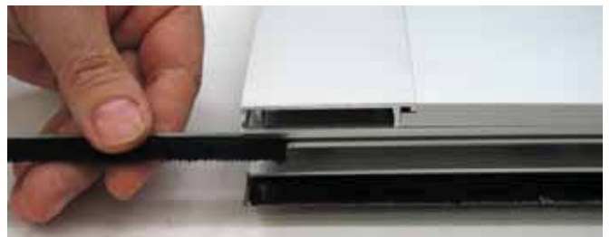
4.6 Insert the brushes SPAZ14 as shown in the diagram, and block them to prevent them from sliding.
