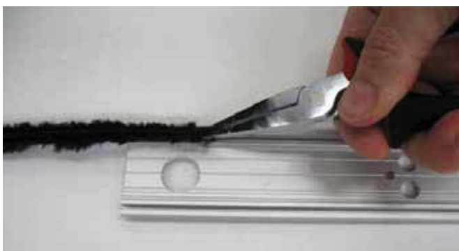
4.10 Insert the brush SPA4811 into profiles 3924 and 3820, as shown in the diagram, and block it to prevent it from sliding.
