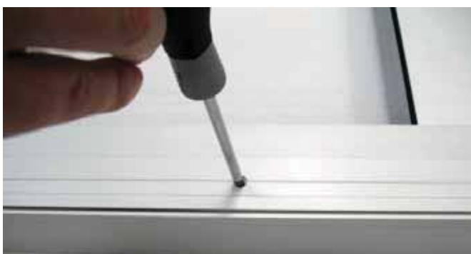
1.23 Attach profile 3831 to the PAM45M profile 3808, or else to the PAM45L profile 3821, as shown in the diagram.
