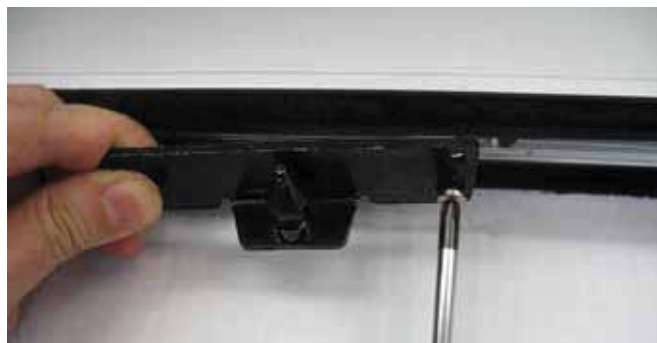
4.12 Fasten detail [4] to profile 3924, as shown in the diagram. Note: Be sure to take note of the wing's opening direction.
