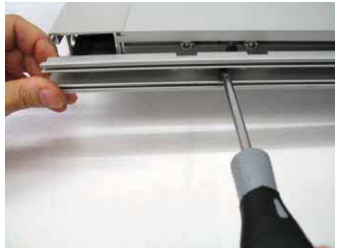
1.5 Fasten profile 3805 to the lower portion of the wing, as shown in the diagram.
