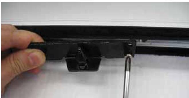
2.17 Fasten detail [16] to profile 3924, as shown in the diagram. Note: Be sure to take note of the wing's opening direction.
