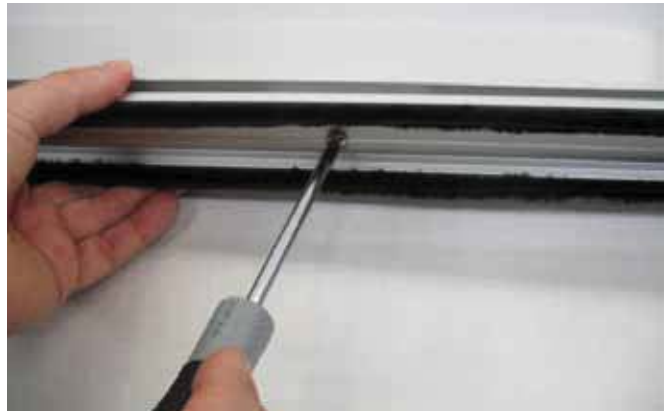
1.11 Fasten profile 3924 to the upper portion of the wing, as shown in the diagram.
