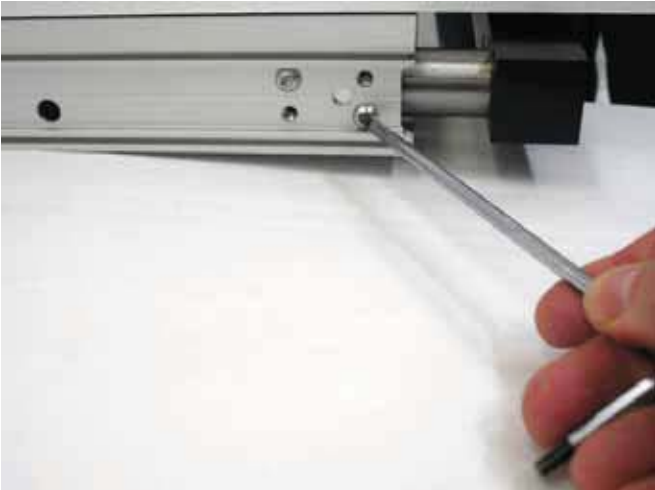
1.9 Fasten detail [3] by tightening the eight fastening screws, as shown in the diagram.
