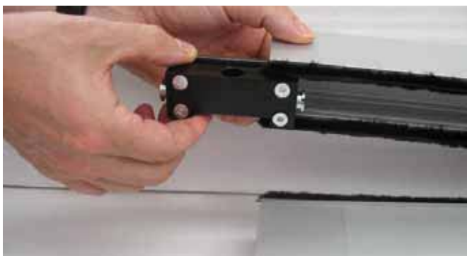
6.17 Insert detail [5] into profile 3820, as shown in the diagram. Note: Be sure to take note of the wing's opening direction.
