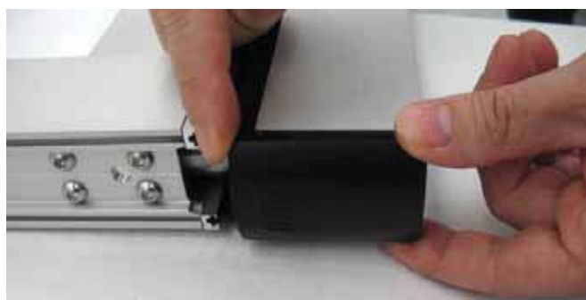
1.19 Insert detail [6] into profile 3820 near detail [3], as shown in the diagram.
