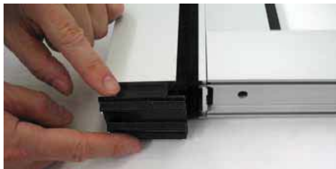
1.21 Insert detail [7] into profile 3820, as shown in the diagram.
