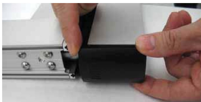
4.19 Insert detail [6] into profile 3820 near detail [3], as shown in the diagram.
