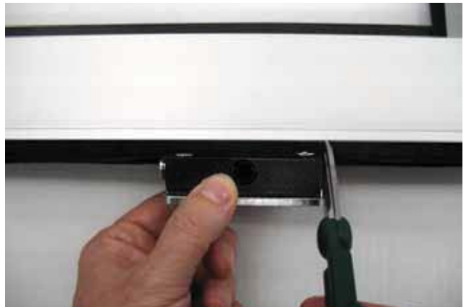
1.13 Trim the brush SPAZ4811 where it connects with detail [5], as shown in the diagram. Note: Be sure to take note of the wing's opening direction
