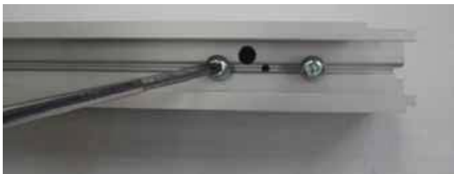
1.3 Insert detail [1] into the PAM45M profiles 3800 and 3813 or else the PAM45L profiles 3599 and 3822, and fasten it as shown in the diagram.
