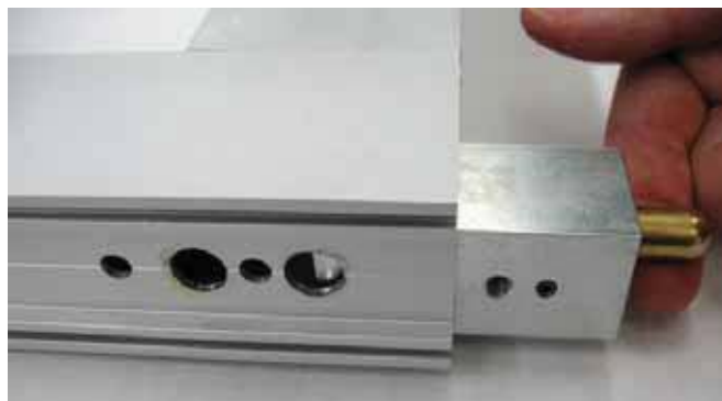
2.4 Insert detail [11] into the lower portion of the wing and fasten it as shown in the diagram.
