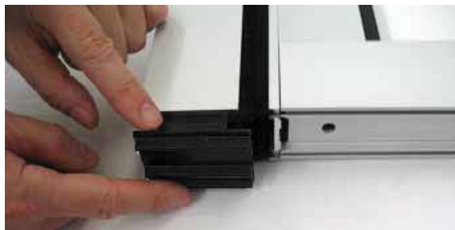
6.21 Insert detail [7] into profile 3820, as shown in the diagram.
