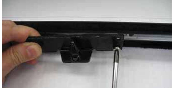
1.12 Fasten detail [4] to profile 3924, as shown in the diagram. Note: Be sure to take note of the wing's opening direction.
