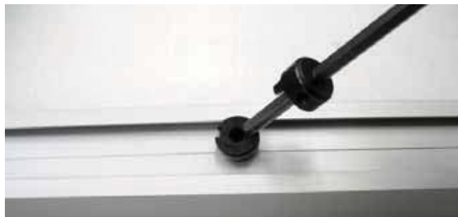
2.20 Fasten the expanders [18] to the perimeter profiles 3809, as shown in the diagram, using the appropriate 6 mm Allen key.
