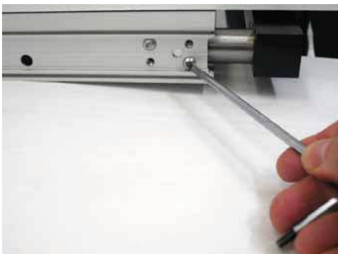
4.9 Fasten detail [3] by tightening the eight fastening screws, as shown in the diagram.
