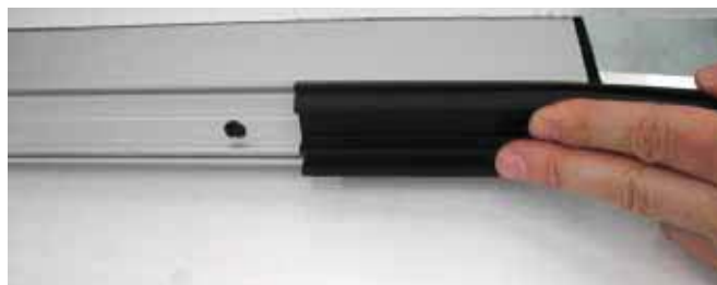
6.20 Insert the seal 3837 onto the PAM45M profile 3808, or else the PAM45L profile 3821, as shown in the diagram.
