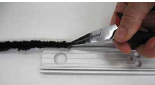
1.10 Insert the brush SPAZ4811 into profiles 3924 and 3820, as shown in the diagram.
