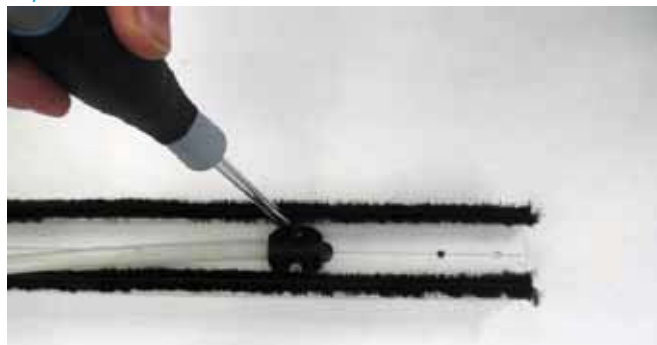
2.21 Fasten detail [19] to profile 3809, as shown in the diagram.
