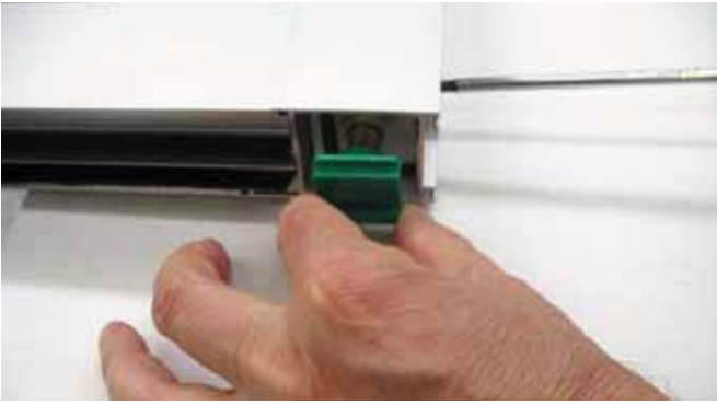
1.7 Insert detail [2] into the lower portion of the wing and fasten it as shown in the diagram.
