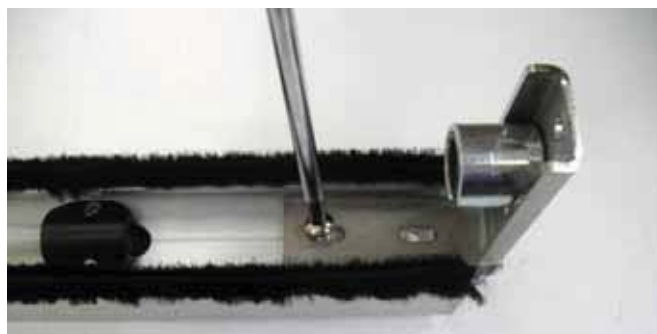
2.23 Fasten detail [21] to the upper portion of profile 3809, as shown in the diagram.
