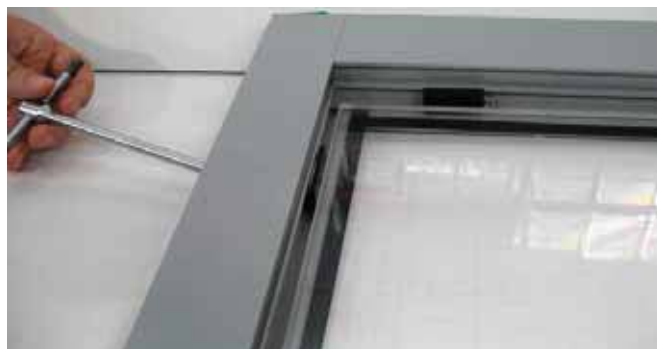
1.26 With PAM45M profiles, insert the glass [9] into the mobile wing, as shown in the diagram.
