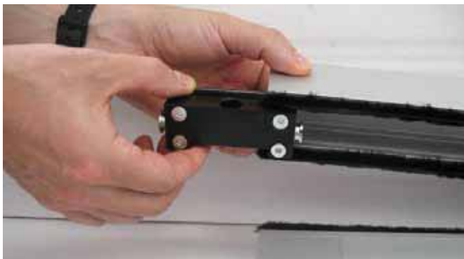
1.17 Insert detail [5] into profile 3820, as shown in the diagram. Note: Be sure to take note of the wing's opening direction
