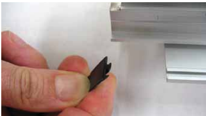
2.1 Insert the seal 3839 into the PAM45M profiles 3800, 3808 and 3813 or else the PAM45L profiles 3599, 3821 and 3822, as shown in the diagram.
