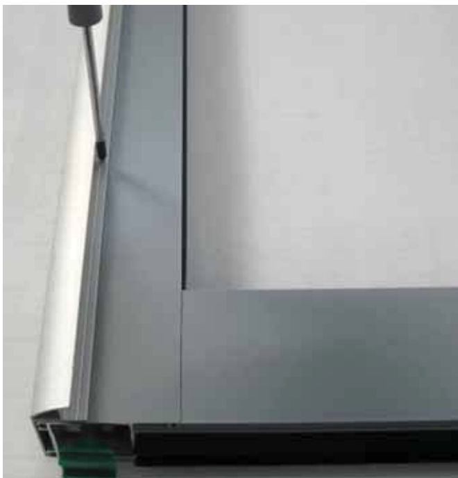
4.23 Attach profile 3925 to the PAM45M profile 3808, or else to the PAM45L profile 3821, as shown in the diagram.
