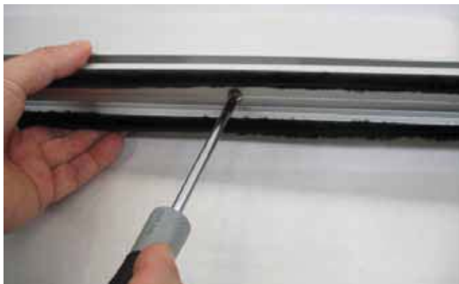
6.11 Fasten profile 3924 to the upper portion of the wing, as shown in the diagram.
