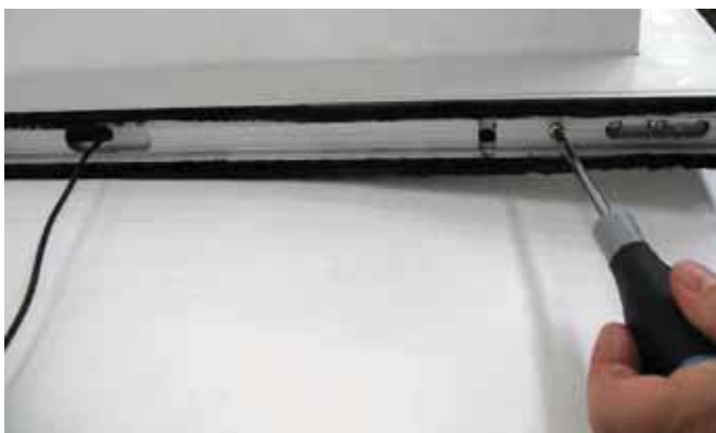
2.18 Fasten profile 3924 to the hinge side vertical upright, as shown in the diagram.
