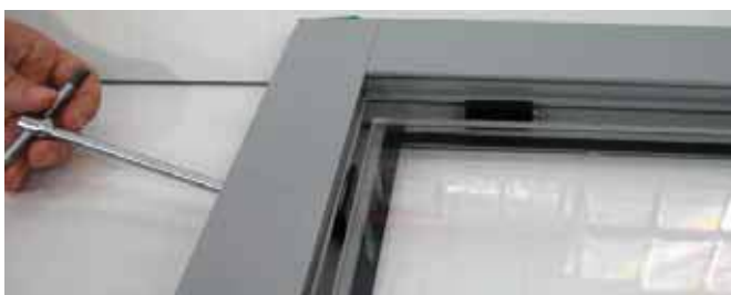
4.24 With PAM45M profiles, insert the glass [9] into the mobile wing, as shown in the diagram.
