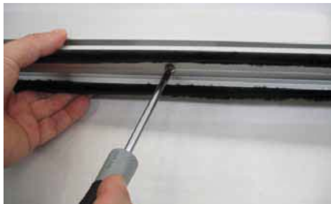
4.11 Fasten profile 3924 to the upper portion of the wing, as shown in the diagram.
