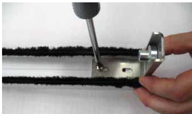
2.22 Fasten detail [20] to the lower portion of profile 3809, as shown in the diagram.
