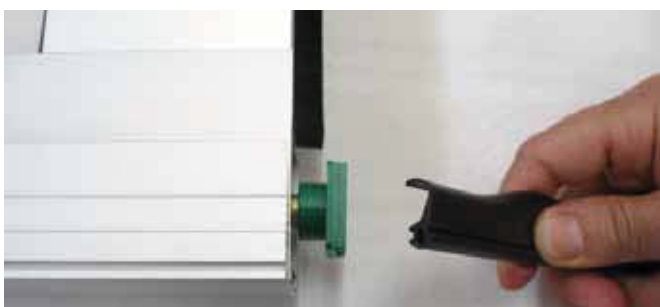
1.24 Insert seal 3838 into profile 3831, as shown in the diagram, and block it to prevent it from sliding.
