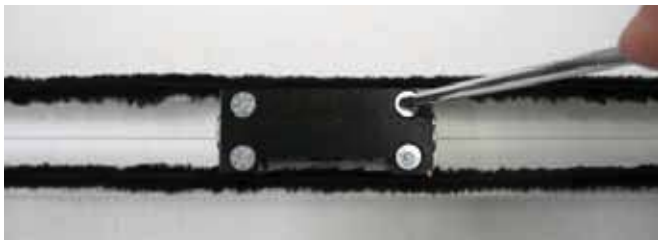
2.24 Fasten detail [22] to profile 3809, situated above the wing, as shown in the diagram.
